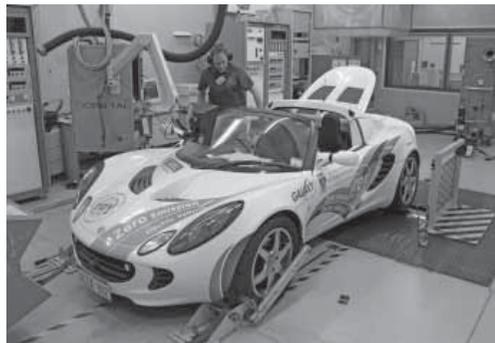
The EV Lotus Elise is tested on Orbital Engines' dynamometer
